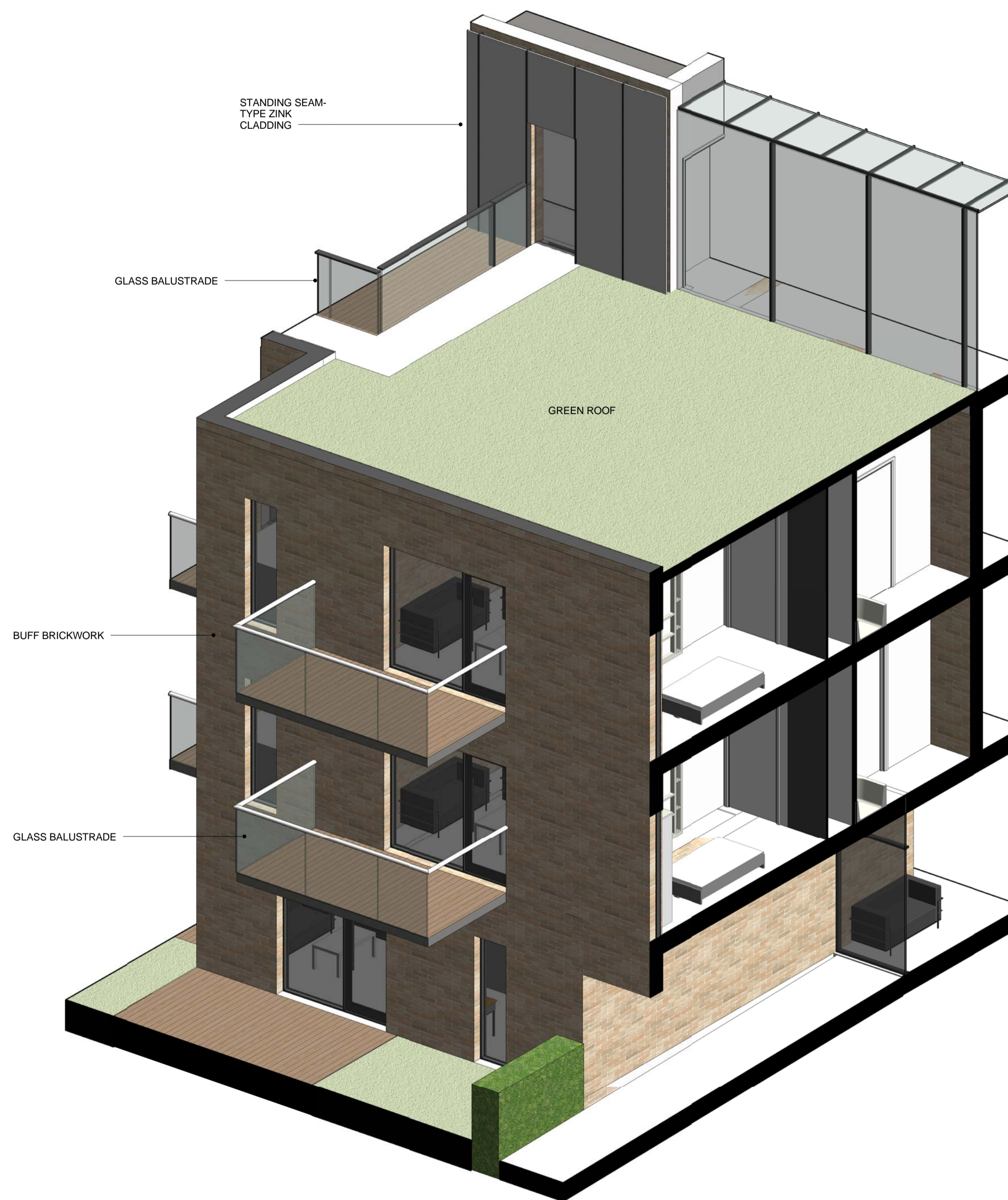
1 SECTIONAL 3D VIEW OF WEST FACADE
