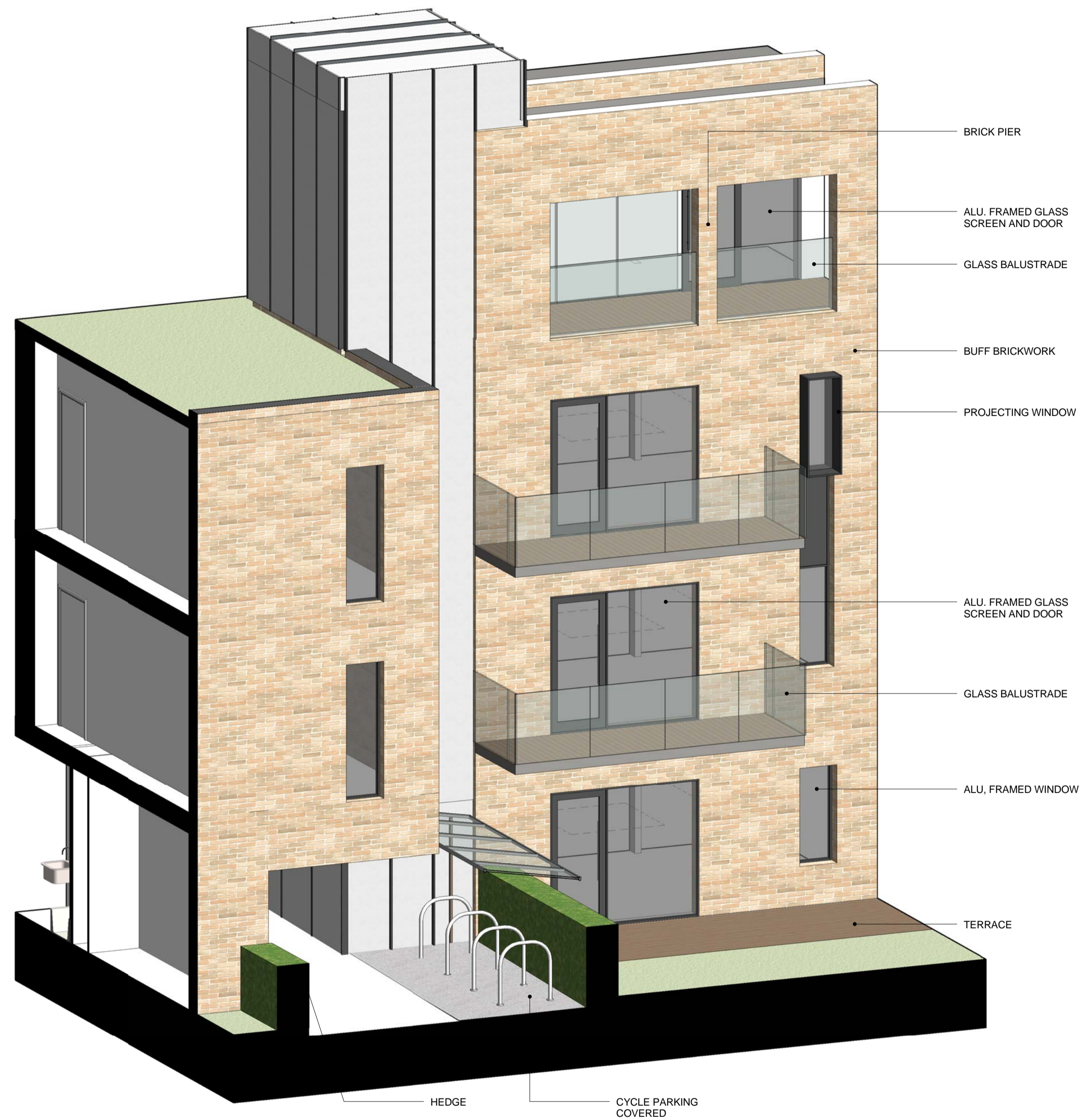
4 SECTIONAL 3D VIEW OF WEST FACADE
